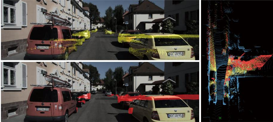
**Fig. 6.** Comparison of  $T$ -frame blind spot and “ground truth” obtained from LiDAR data. Top-left and bottom-left figures show the ground truth and  $T$ -frame blind spots, respectively. Right figure shows the 3D projection of ground truth (yellow) and  $T$ -frame blind spots (red) to LiDAR scan (blue). The green cross indicates the camera position.
