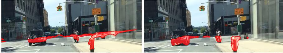
**Fig. 8.** Failure example. Left:  $T$ -frame blind spot (“ground truth”) from a frame in BDD-RBS. Right: Blind spot estimation results from BlindSpotNet trained on BDD-RBS. Due to the bias of BDD-RBS, which lacks left and right turns at intersections, BSN cannot estimate the blind spots caused by the intersection. We plan to address these issues by employing a panoramic driving video for pre-training.
