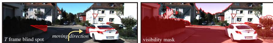
**Fig. 4.** Visibility mask. Left: If the vehicle makes a turn, the blind spots straight ahead across the intersection never become visible. Right: To allow networks estimate such blind spots, we prepare a mask image to indicate the visible area for each frame.
