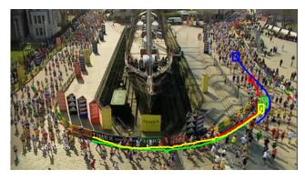
Figure 7. Scenes that lack temporal variations in motion, such as the one shown here from the data set used in [1], exhibit a single motion vector at each spatial location. Such scenes are special cases of reduced complexity that can easily be handled with our approach. The superimposed trajectories show successful tracking of individuals in the scene.
