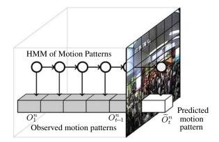
Figure 2. Following [10], the video is subdivided into local spatiotemporal volumes and an HMM is trained on the motion patterns at each spatial location to capture the steady-state motion of the crowd. Using the trained HMM and previously observed motion patterns  $O_1^n, \ldots, O_{t-1}^n$ , we predict the motion pattern  $\tilde{O}_t^n$  that describes how a target moves through the video.
