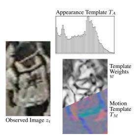
Figure 4. The pedestrian's appearance template  $T_A$  and motion template  $T_M$  are represented by a color histogram and an image of spatio-temporal gradients, respectively. The observed frame  $z_t$  is used to estimate the motion model's error at each pixel, illustrated by the weight image w. The pedestrian's natural movement causes lower weights in moving areas such as the head and shoulders. Pixels behind the pedestrian also change significantly as indicated by the dark background area.
