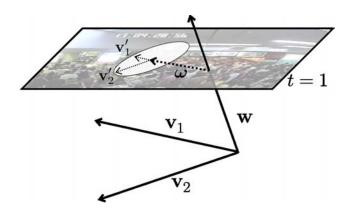
Figure 3. The 3D optical flow w is estimated from the predicted structure tensor matrix as the eigenvector with the smallest eigenvalue. The 2D optical flow  $\omega$  is its projection onto the plane t = 1, representing the predicted movement of the subject through the cuboid. We estimate the optical flow's variance by projecting the other two eigenvectors  $v_1$  and  $v_2$  onto the same plane, and scaling them with respect to the estimation confidence.
