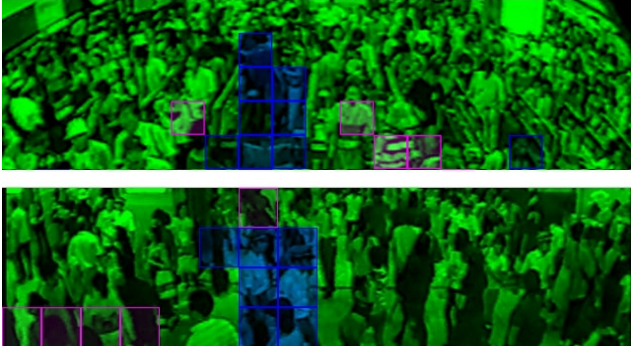
Figure 6. Detection of unusual motion patterns in the concourse video (top) and the ticket gate (bottom). Correctly classified unusual cuboids are highlighted in blue, usual cuboids in green, false negatives in red, and false positives in magenta. The intensity of magenta blocks indicates the severity of false positives. Individuals reversing direction and moving in irregular patterns are correctly classified as unusual.
