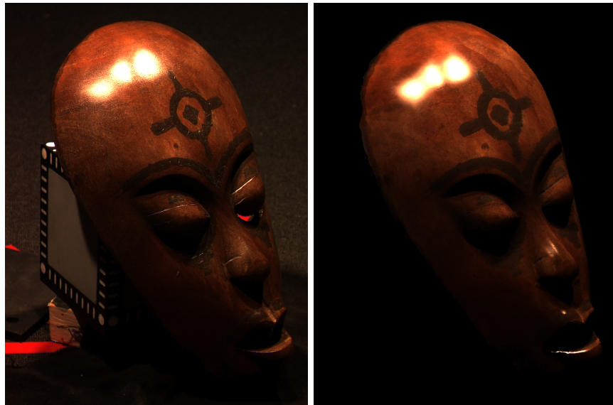
Fig. 10. Comparison between a synthetic image from a novel viewpoint and a real photograph. Left: real photograph, Right: synthetic image.
