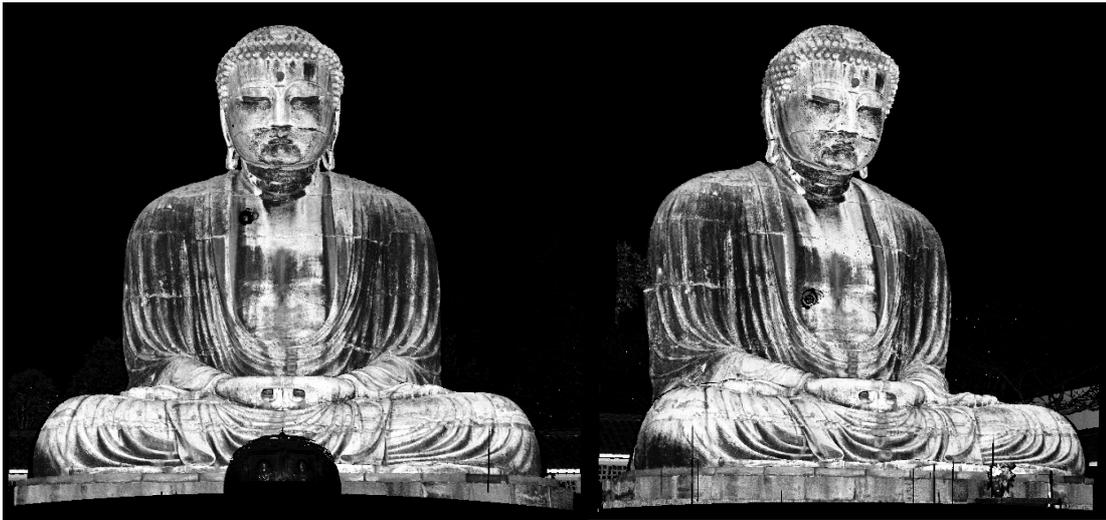
Figure 2.4: Images using laser reflectance strength as pixel values.
