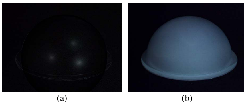
Fig. 10. Reflection components separated from Figure 9 (a). (a) Specular reflection image. (b) Diffuse reflection image.
