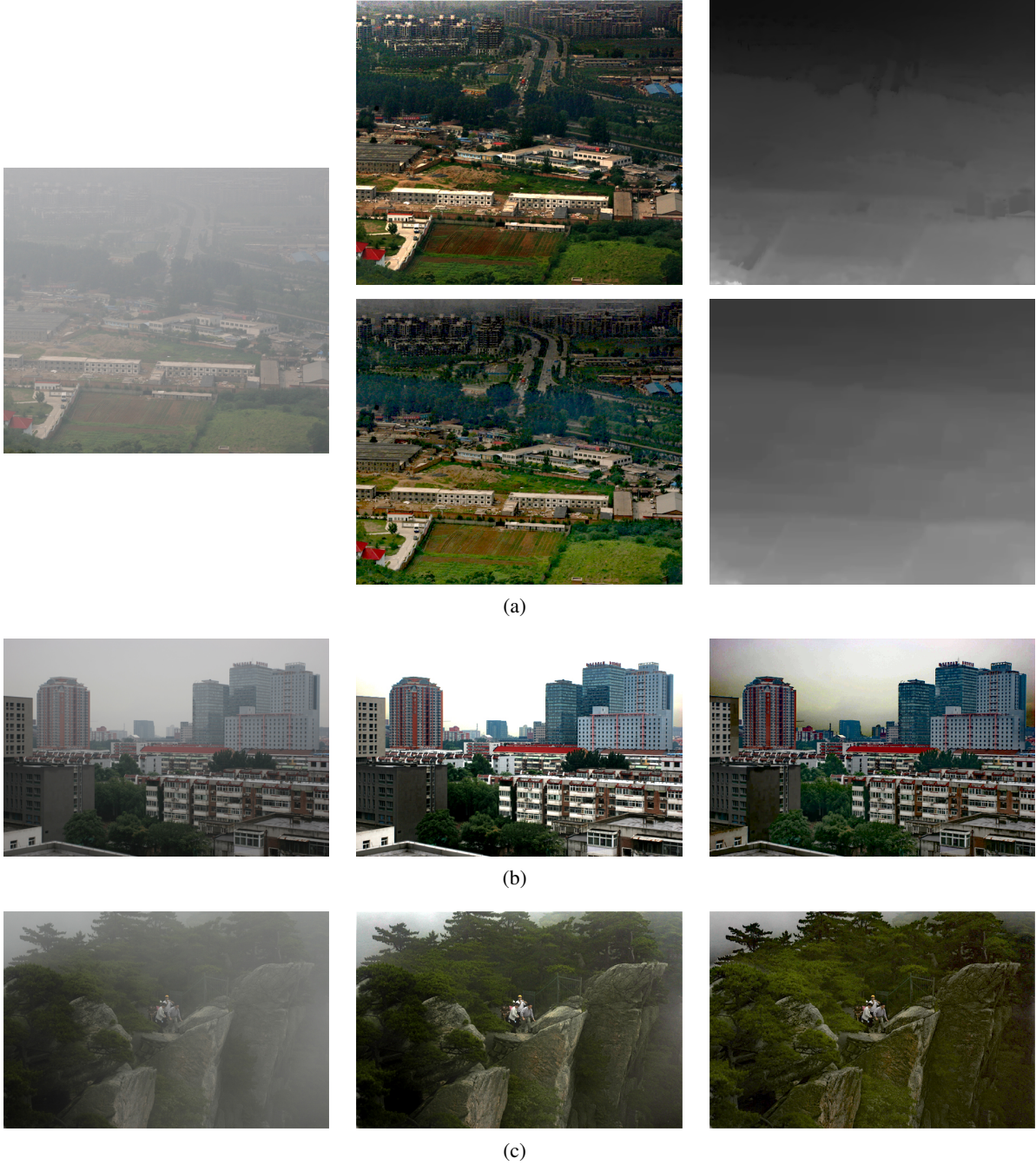
Fig. 8. Factorization results of real-world foggy images, of (a) an aerial city view, (b) an urban view, and (c) a cliff, compared with those of another method by He et al (2009b). For the example in (a), in the columns, the input foggy image (left), the estimated albedo image (middle), and the estimated depth image (right) are shown; and in the rows, the results by He et al (2009b) (top), and by our method (bottom) are shown. For the examples in (b) and (c), the input image, the albedo image by He et al (2009b), and the albedo image by our method are shown from left to right, respectively. Overall the factorization results are of similar quality, but our method achieves clearer defogging on particularly challenging scenes like that in (c). The input images and the corresponding results by He et al (2009b) are reprinted from (He et al, 2009a).
